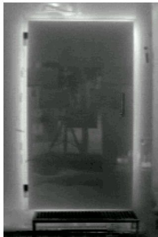
Figure 3.2c. Infrared picture of the test cell door.
