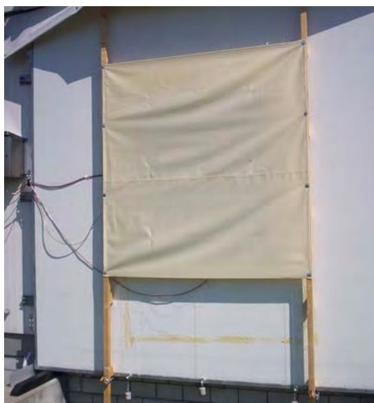
Figure 7.1. Photograph of the exterior shade mounted on the test cell.
