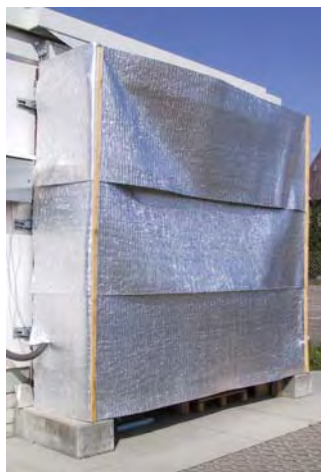
Figure 4.1a. Photograph of test toom with external chamber.
