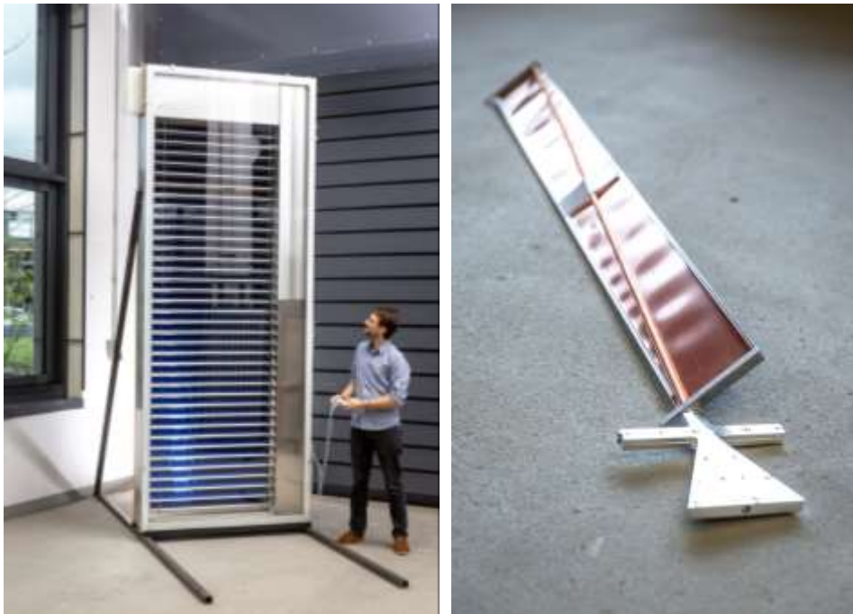
Figure 2-65: Left: Test sample of double skin facade element (3.6 m x 1.4 m) with integrated solar thermal venetian blind seen from the exterior side. Right: Back surface of a slat with diagonally mounted heat pipe and triangular adapter in the foreground (back cover sheet removed). © Fraunhofer ISE
