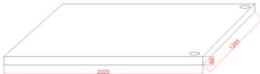
Figure 3.2.3: Principle sketch of the first heat storage module with two holes used to fill in the salt water mixture.
