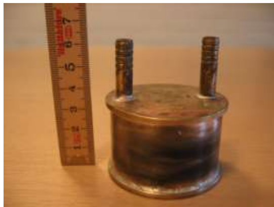
Figure 3.2.11: Brass tank with CO 2 used for starting the solidification.
