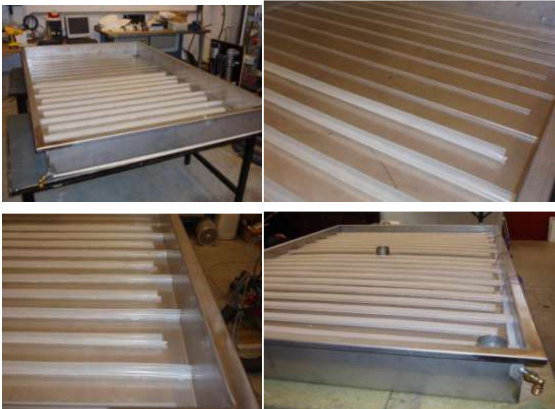
Figure 3.2.6: Photos of the first heat storage module with silicone pipes attached to the upper surface.
