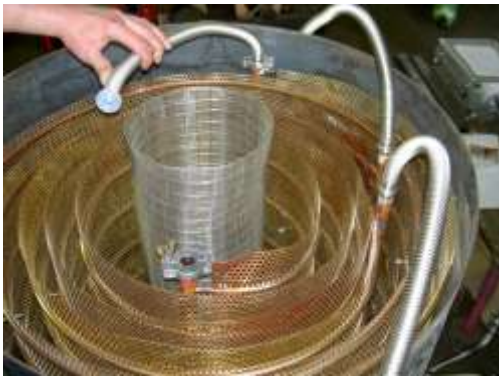
Figure 3.3.4: Spiral heat exchanger made from perforated sheet copper, source: AEE INTEC, Austria.
