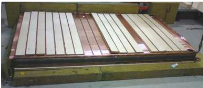
Figure 3.2.4: Principle sketch of the first heat storage module with heat transfer system and insulation.
