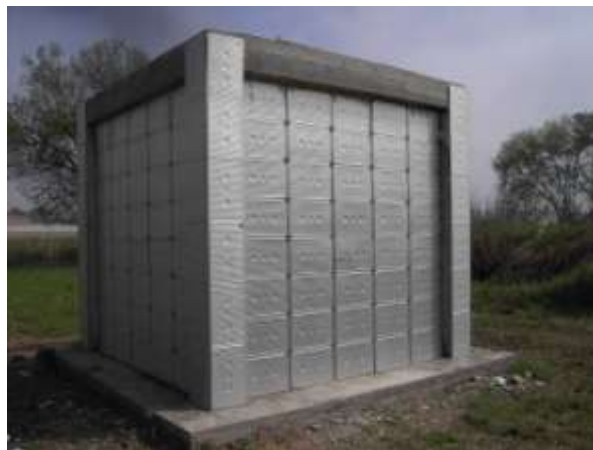
Figure 3.4.4: Conventional brick cubicle with macroencapsulated PCM.
