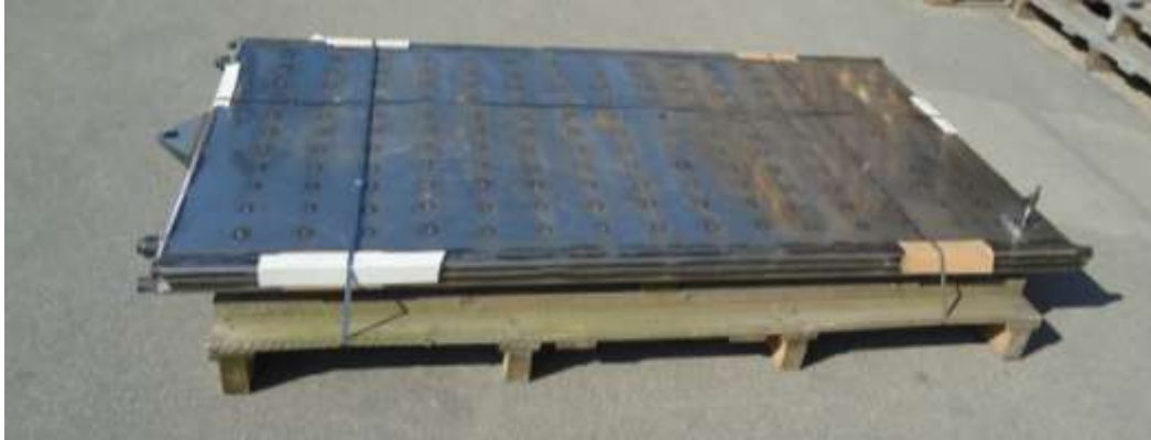
Figure 3.2.10: Photo of the third heat storage module with two holes at the left hand side of the module used to fill in the salt water mixture.
