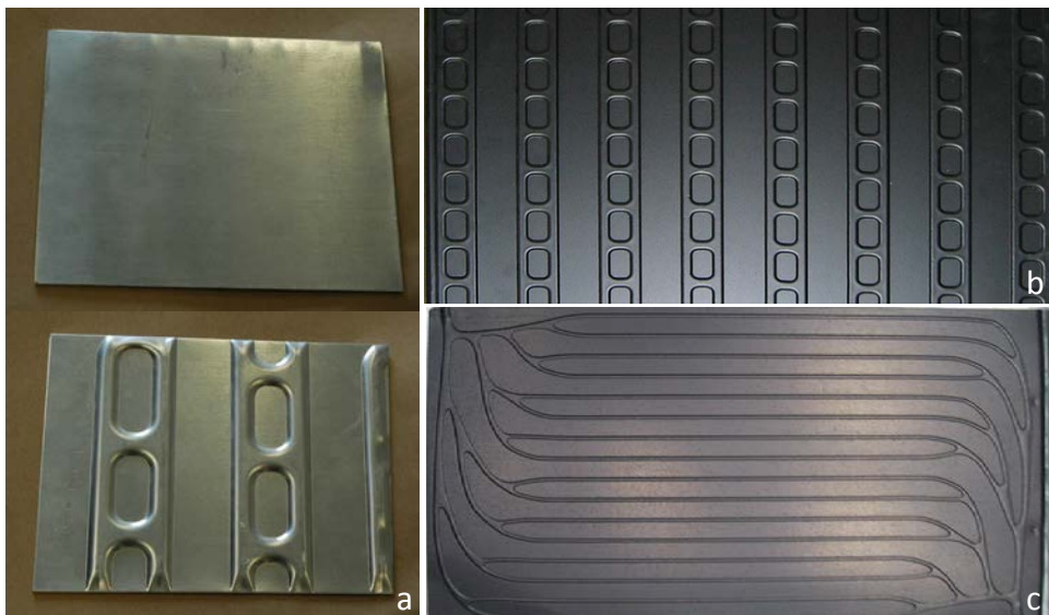
Fig. 3.2-10a: Two faces of a roll-bond “single blow” sample: back face with visible piping pattern, front face flat (pict. EPFL-LESO).
