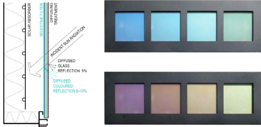
Fig. 3.1-19 left: Principle of coloured filter and diffusion layer.
