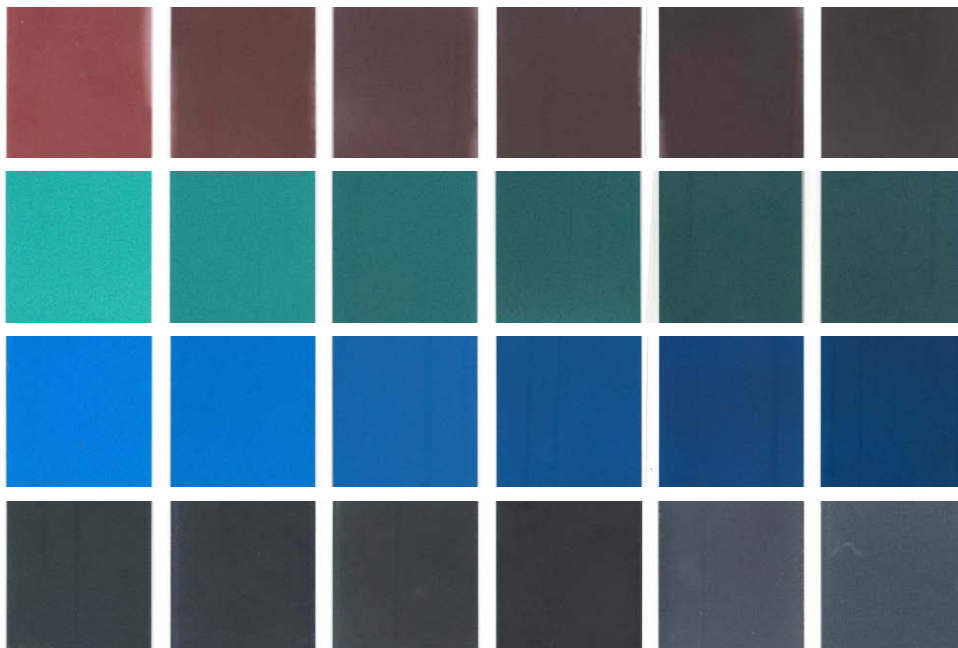
Fig.3.2-6: Thickness insensitive spectrally selective paints (TISS) palette developed at the National Institute of Chemistry Ljubljana, Prof. Boris Orel, within EU project Solabs.
