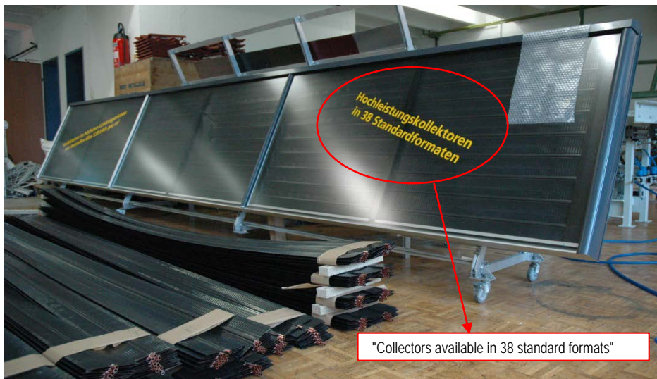
Fig. 3.1-14: Winkler glazed collectors system for facade: available in 38 “standard” formats.
