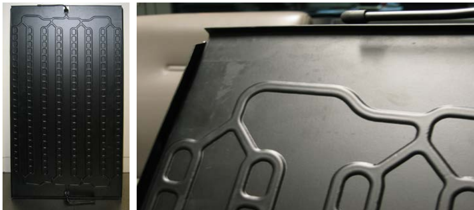
Fig. 3.1-15 a: Solar absorber prototype with hydraulic system using the roll bond technology.
