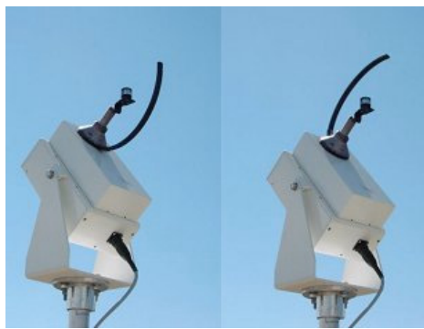
Figure 1: One example for a RSI: Rotating Shadowband Pyranometer (RSP) in normal position (left) and during rotation (right).
