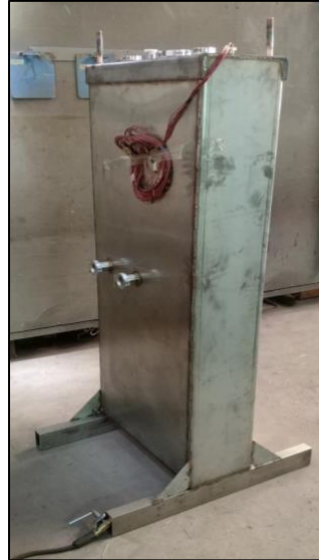
The first prototype, ready for tests. It contains about 250 liters of salt.
