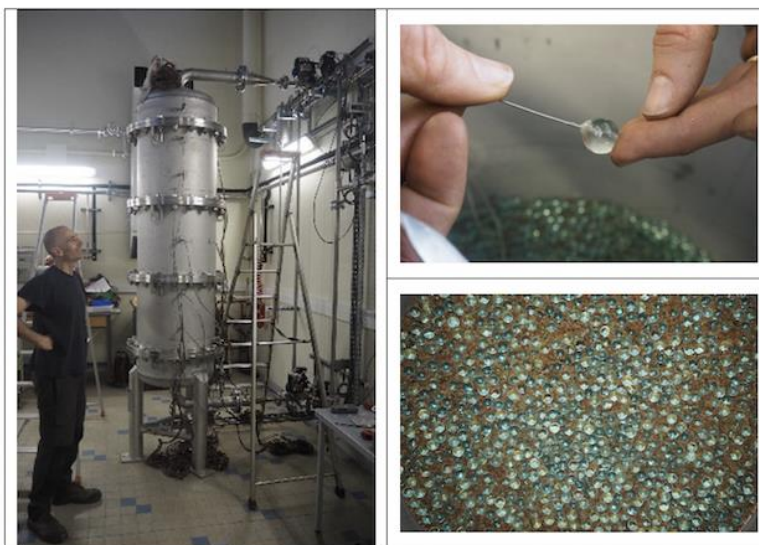
Photos of the storage module before insulation (left), thermocouple in glass sphere (upper right) and bed of glass spheres and silica gel (bottom right).
