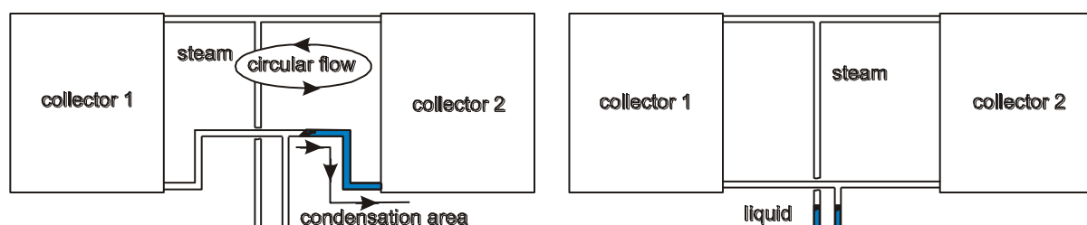
Figure 19: Connection of collectors leading to a) poor emptying behaviour, b) good emptying behaviour (Hausner & Fink, 2000).
