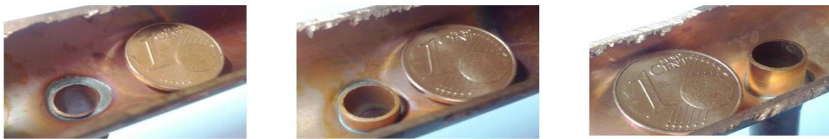
Figure 5: Examples of different penetration depths of the absorber pipe into the collector manifold pipe, as commonly found on the market (Philip Ohnewein, 2013).
