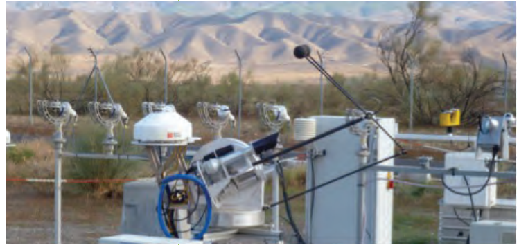
▲ Figure 2. Solar tracker with reference radiometers for RSI calibration at Plataforma Solar de Almería.
