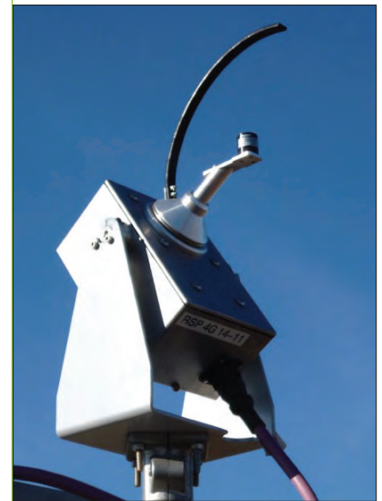
▲ Figure 1. Rotating Shadowband Irradiometer (RSI) in normal position (left) and during rotation (right).
